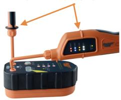
Check the correct function of the VIP ESI both before and after use with a true AC output proving unit such as the Socket and See SP400.
